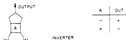
Figure 10. The wiring diagram of one molecule to obtain an "INVERTER".
